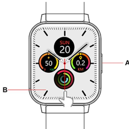
**Button A:** Hold to switch ON/OFF, tap/press to turn ON/OFF the screen.
